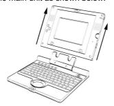
Attach the screen to the main unit as shown below:
